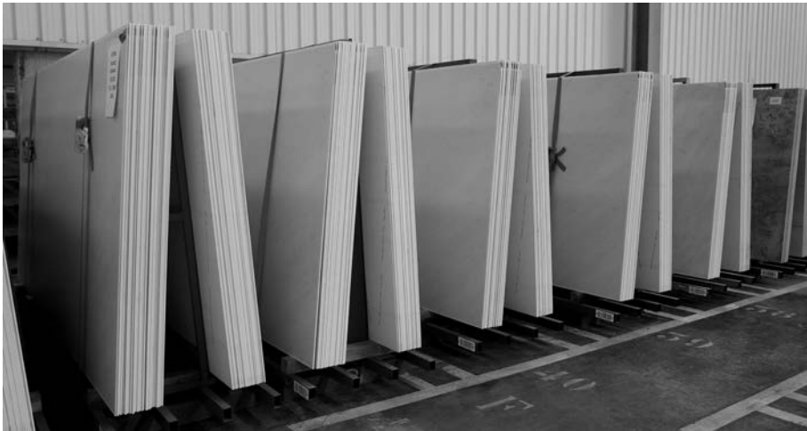
Storage of Neolith slabs in the shop
