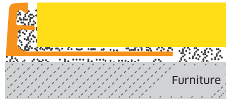
■ Cross-sectional image of a Jolly- AC profile
