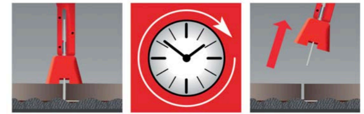
Tension until level Wait for glue to dry Remove strap and cap
