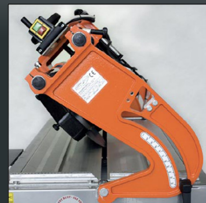
45 DEGREE TILT FOR MITRED AND ANGLED CUTS
