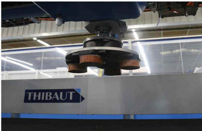
Polishing with Frankfurt flexible plate
