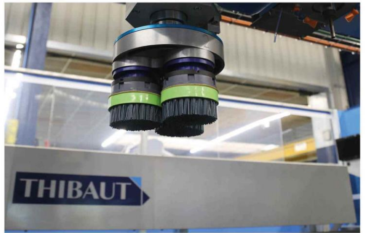
Brushing with AR-3 satellite head
