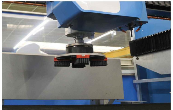
Brushing with Frankfurt flexible plate
