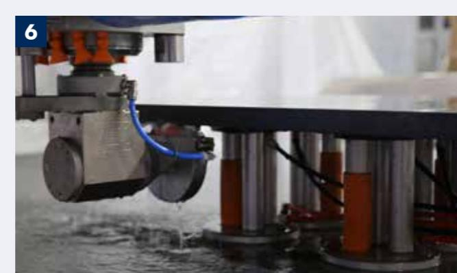
**EN Angle drive for underneath groove (available on 4-axis versions)**
