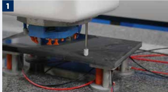
**EN Slab sensing device**
