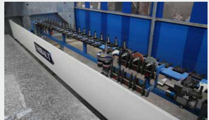
**EN 47 positions linear tool magazine. It is possible to equip the machine with 2 magazines ( $47 \times 2 + 1 = 95$  tools).**
