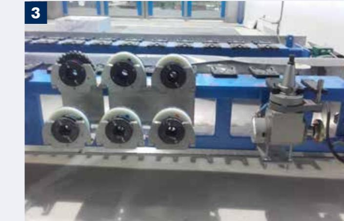
**EN Modulo and tool magazine for edges polishing with Modulo**
