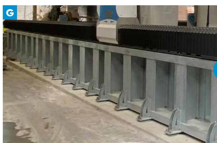
**EN** Welded structure plinths
