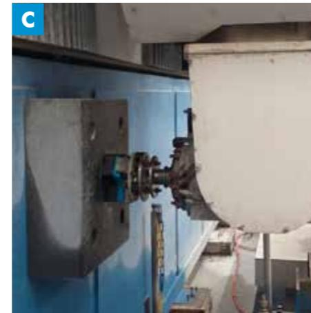
**EN** Polishing head sensor device
